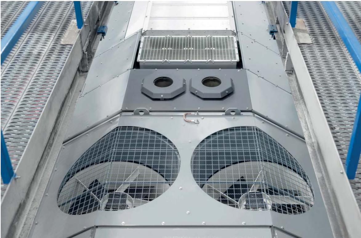
Roof cooling unit for locomotive
