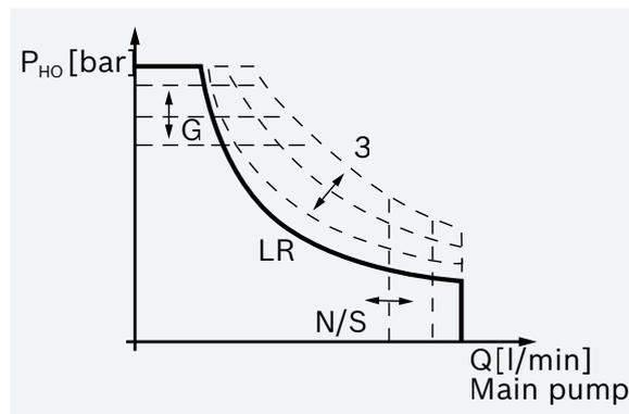
Figure 1: Pump control functions
